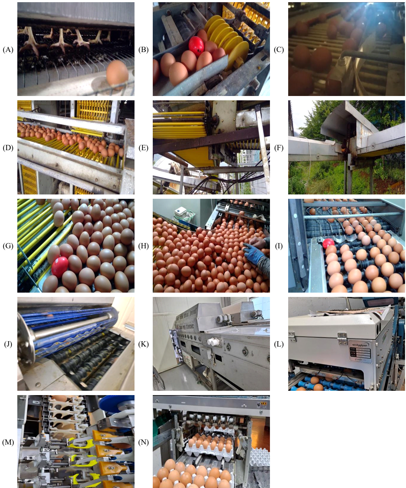
Fig. 2. Egg transit system from laying house to egg packing center. Electronic egg (red in color) is shown in B, G, and I. A: cage with egg belt; B, C: elevator; D, E, F: conveyor; G, H: accumulator; I, J: connector; K: egg washer and dryer; L: crack detector; M: transfer; N: packer.
